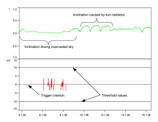
Figure 4: Typical monitoring results from the damaged pier
