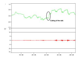
Figure 5: Inclination during cutting of the rails
